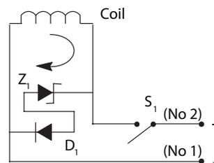
NOTE: These surge suppression devices are "Polarity Dependent." Proper biasing conditions must be met when installing/connecting a coil in a system. Times represent cessation/application of voltage to coil versus velocity (start/stop) of a cylinder using a single solenoid, spring offset valve (time in milliseconds).
