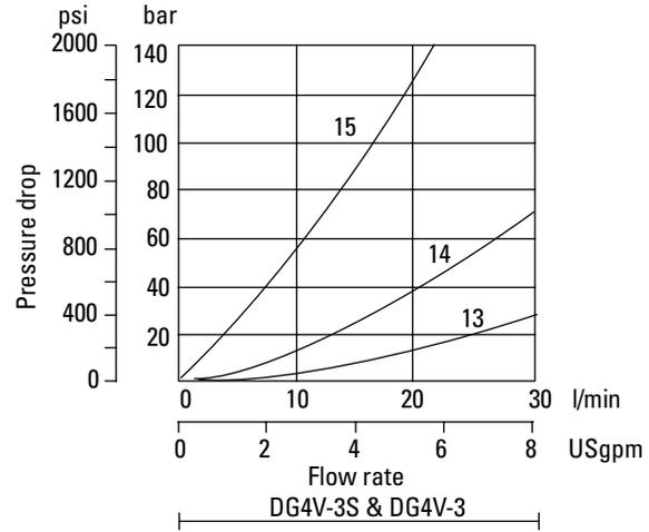
▼ Curve for spool type 6: not recommended for flows in excess of 60 l/min (15.8 USgpm).
